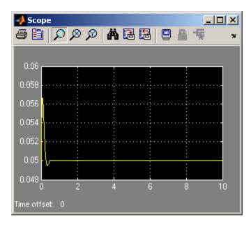
As you can see, the system is now stable and the height of the magnetic ball settles at the desired height of 0.05 m.
