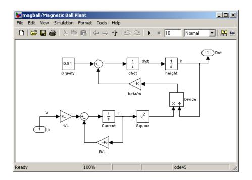
The input to the Magnetic Ball Plant system, which is also the output of the Controller subsystem, is the voltage, V. The output is the height of the ball, h. The system contains three states within the three integrators: height, dhdt, and Current.
