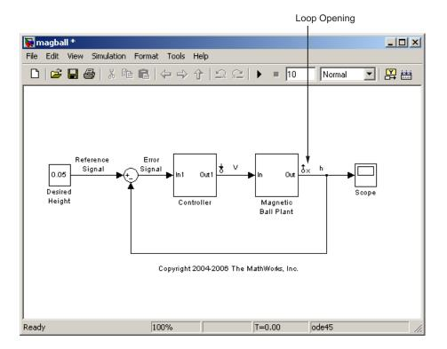
**Note** You do not need to place a loop opening in the same place as an input or output point. For example, in the following figure the highlighted blocks are included in the linearization. The loop opening is placed after the gain on the outer feedback loop, which removes the effect of this loop from the linearization. Placing a loop opening at the same place as the output point would have removed the effect of the inner loop from the linearization as well.
